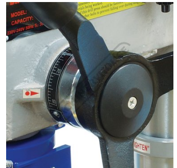
Drilling Depth Stop Setting With Scale
