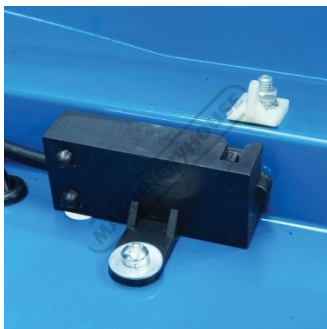
Safety Micro Switch on Pulley Guard
