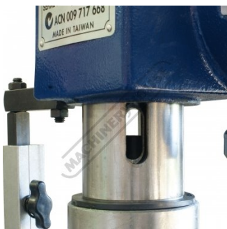
Drill Chuck Set Up For Removal
