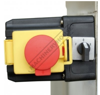
Emergency Stop Switch and Overload Protection
