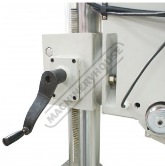
Rack and Pinion Wind Up Drill Head
