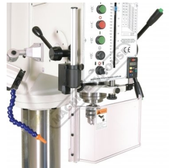
Interlocked Spindle Safety Guard
