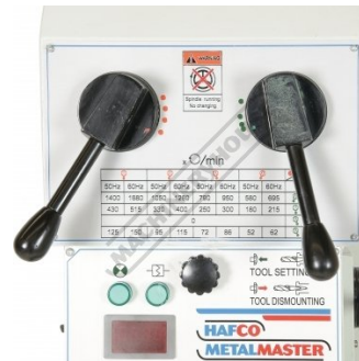
Drill Speed Selection Levers & Speed Chart
