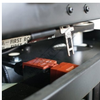
Micro Switch on Belt Cover
