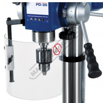
Drill Chuck Safety Guard With Micro Switch
