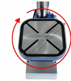
Cast Iron Table Rotates 360 Degree
