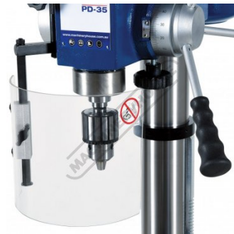
Drill Chuck Safety Guard With Micro Switch
