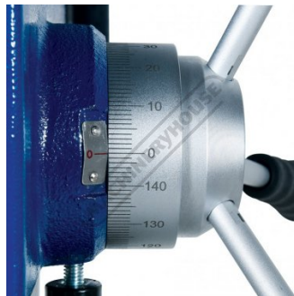
Drilling Depth Stop Setting With Scale
