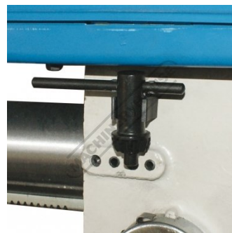
Chuck Key Mounted to side of Head
