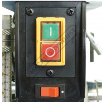
Magnetic Switch and Light Switch
