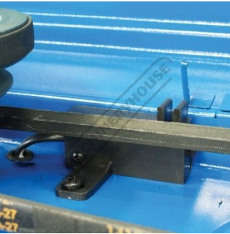
Safety Micro Switch on Pulley Guard
