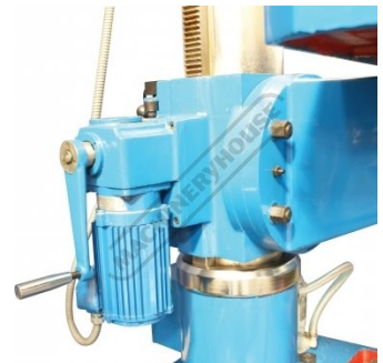
Motorised Rise and Fall Work Table
