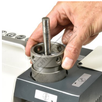
Grinding Split Point Station
