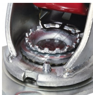
Ball Bearing Base With Greasing Nipple
