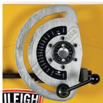
Top Tool Height Adjustment Scale & Lock
