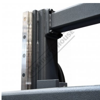
Linear Guide Ways on Posts
