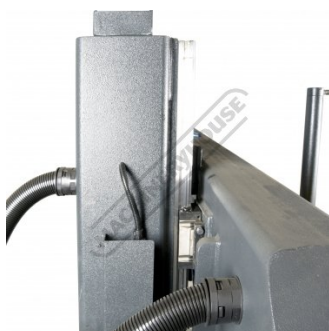
Linear Guide Ways for Improved Accuracy
