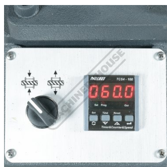
Head Lock Switch with Digital Mitre Angle
