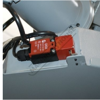
Safety Blade Guard Micro Switch
