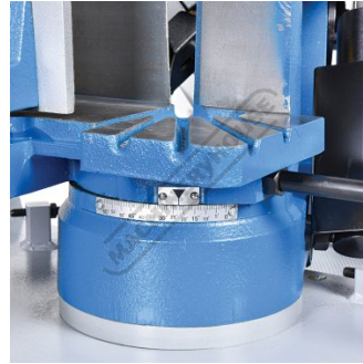
Swivel Head with Scale up to 60 Degree
