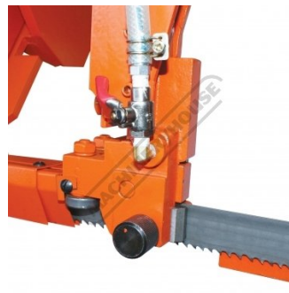
Ball Bearing Blade Guides with Carbide Pads
