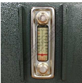
Hydraulic Oil Level Gauge
