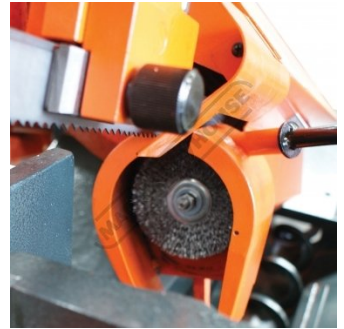
Wire Wheel Blade cleaning Brush
