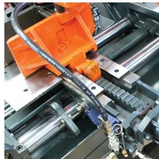
Quick Action Vice on Rack Type System
