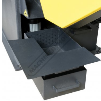
Coolant Pump Reservoir with Swarf Trap
