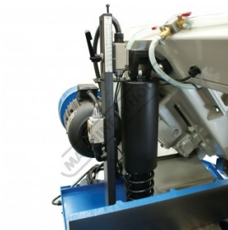
Rear Hydraulic System
