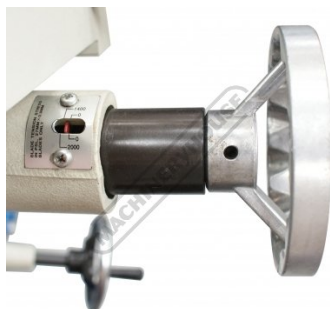
Blade Tension Gauge
