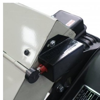
Blade Guard Safety Micro Switch
