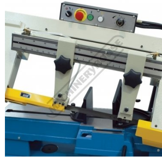
Quick Adjustment Blade Guide System
