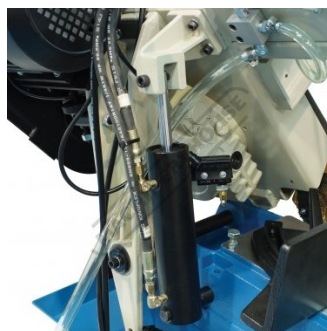
Hydraulic Arm With Automatic Cut Out Switch
