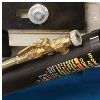
Hydraulic Ram Down Feed Control
