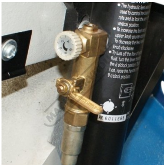
Down Feed Control
