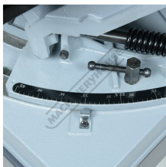
Swivel Head Scale Set at 30 Degrees
