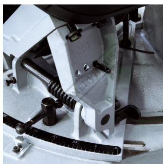
Adjustable Spring To Set Cutting Beam Force
