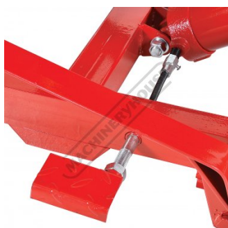
Lever To Lower Platform
