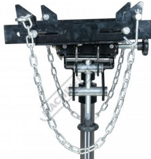
Saddle Plate Lateral Movement Left 35mm
