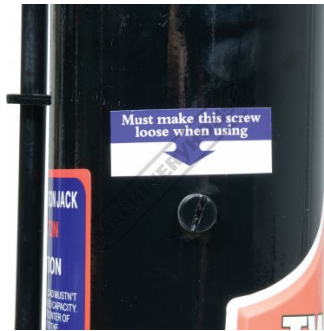
Air Bleed Release Screw
