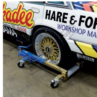
Positioning Jack in Place 2
