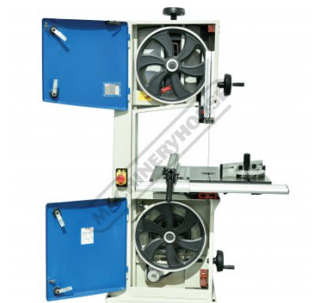
Blade Guards Fitted with Safety Micro Switches
