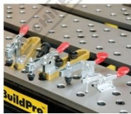
Toggle Clamps Can Be Mounted on Top of the D Stop Bars
