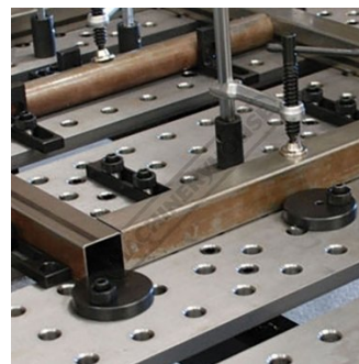
Eccentric Pads can locate or stop stock of varying shapes and is especially useful for stopping round stock
