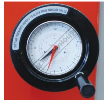
Variable Blade Gap Adjustment Dial
