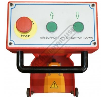
Pneumatic Sheet Support and Emergency Stop on Mobile Foot Control
