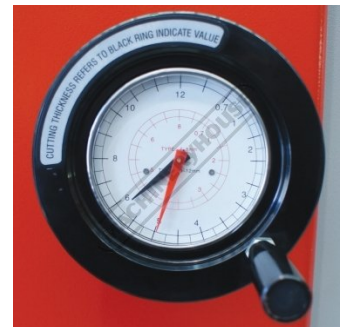
Variable Blade Gap Adjustment Dial
