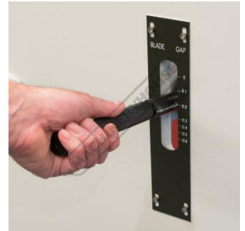
Quick Action Blade Clearance Adjustment Operation
