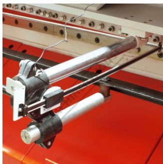
Backgauge Scale for Digital Readout
