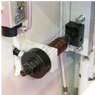
Quick Action Blade Clearance Adjustment
