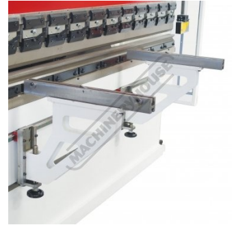
Sliding Front Sheet Supports on Linear Guideways
