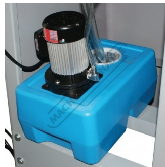
Coolant Pump and Tank
