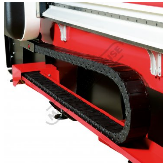
Enclosed Cable Management Close Up
