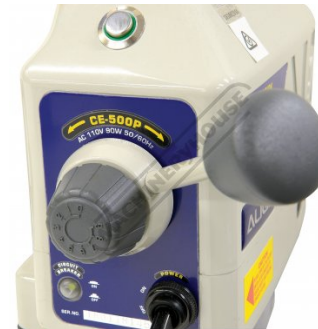
Engagement Lever & Variable Speed Dial
