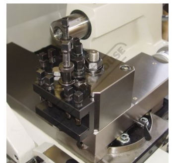
Quick change toolpost with additional holders
