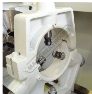
Fixed & travelling steadies with roller bearings
