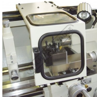
Sliding toolpost guard deflects swarf into tray
