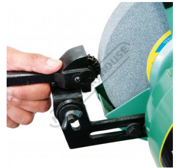
Setup for Dressing a Grinding Wheel Close Up
