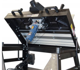
Mounting a Suitable Router
