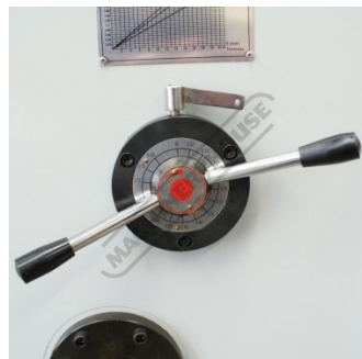
Blade Clearance Adjustment Lever
