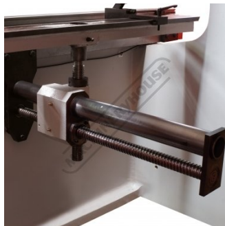
Estun NC E21 Control Ballscrew Back Gauge
