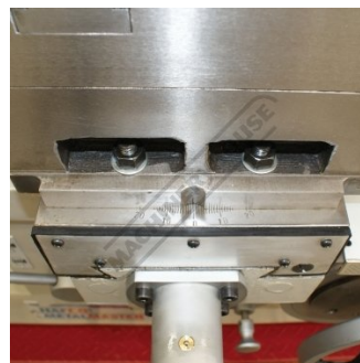
Taper Adjustment on Compound Slide
