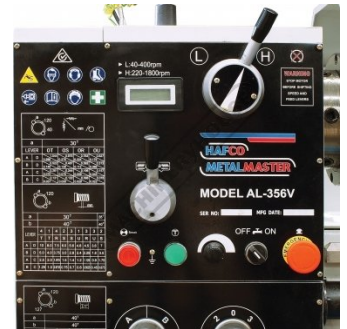
Spindle Speed Controls
