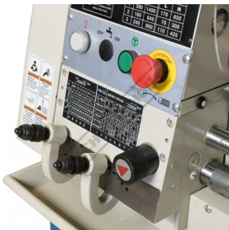
Feed Threading Levers and Control Panel
