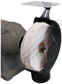
Buffing Wheel Safety Shield and Dust Chute
